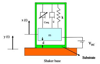
Figure 9. A single-degree-of-freedom model for the capacitive accelerometer.
