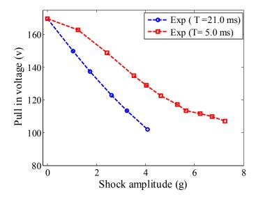
Figure 16. Experimental data of the pull in- shock curves when T = 5.0 ms and 21.0 ms.
