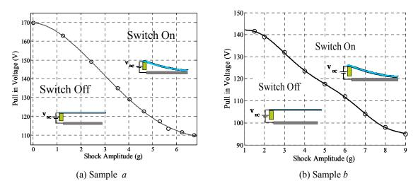
Figure 6. Pull in voltage of the accelerometer against the shock amplitude of a sine pulse of duration T = 5.0 ms.
