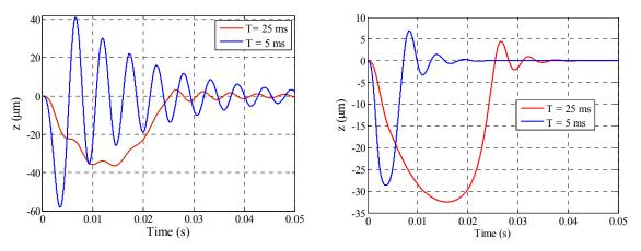
**Figure 14.** A time history for the response of the capacitive accelerometer when actuated by a half-sine pulse amplitude of 5.0 g for the case of (a) no squeeze film damping (b) including the squeeze film damping effect. The figure shows that the quasi-static shock load (T=25.0 ms) effects the proof mass deflection more than the dynamic shock load (T=5.0 ms), in the presence of squeeze film damping.
