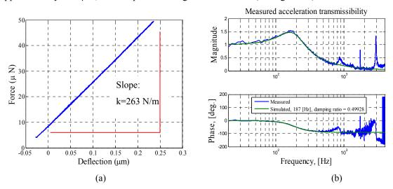
**Figure 10.** Parameter extractions. (a) Force versus deflection curve used to extract the linear stiffness of sample *a* using the nano- indentation machine.(b) Frequency response of the capacitive accelerometer showing the extracted parameters (damping and natural frequency).
