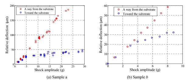
Figure 5. The maximum deflection of the proof mass at different shock levels for the cases when the proof mass moves toward and away from the substrate.
