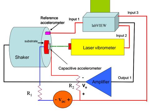
Figure 1c. Schematic for the experimental setup and the data acquisition system.
