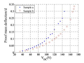
Figure 2. Variation of the absolute value of the proof mass displacement normalized by the gap spacing underneath the proof mass d for various values of the DC bias  $V_{DC}$ .
