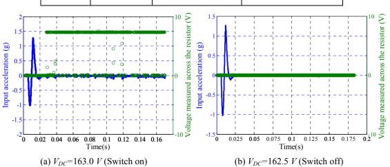
Figure 8. Input acceleration of 1.2 g magnitude, with the voltage measured across the 470  $\Omega$  resistor.
