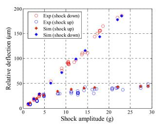
Figure 11. Simulation results (stars) and experimental data (circles) of the proof mass deflection of sample *a* versus shock amplitude when T = 5.0ms.
