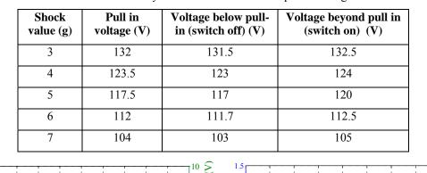
Table 1: Sensitivity of the switch for selected points on Fig.7b
