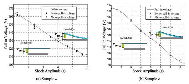
Figure 7. The switch sensitivity to variation in  $V_{DC}$ . Points below the solid line represent the switch in the offposition while points on or above the solid line represent the switch in the on-position.
