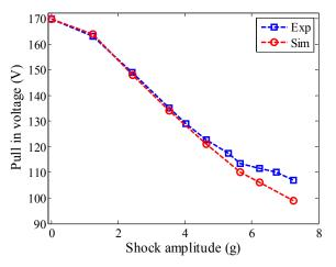
Figure 12: Simulation results (circles) and experimental data (square) for the pull in voltage of sample *a* against the shock amplitude of a sine pulse of T = 5.0ms.
