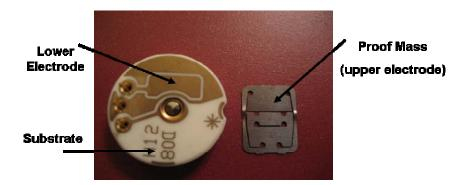
Figure 1a. A picture for a taken-apart commercial-off-the-shelf capacitive accelerometer, fabricated by Sensata Technologies [15], used for testing the shock-threshold switch.
