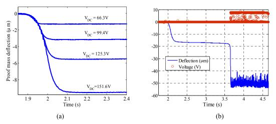
**Figure 3**. The transient response of the proof mass of sample *a* for different voltage values below pull-in (a) and at the pull-in voltage  $V_{DC}$  =169.7 V (b) as monitored by a Laser Doppler Vibrometer (blue). Figure b also shows the reading of the induced voltage across the 470  $\Omega$  resistor (red).
